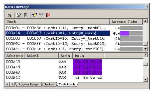
Figure 5.124 Data Coverage window (task stack specification)
